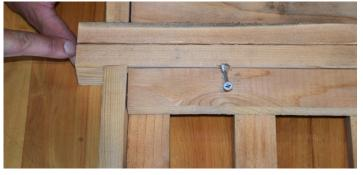
The sticker that says "BOTTOM" should be facing you. Be sure to flush the ends of the 2 panels prior to screwing them together.
