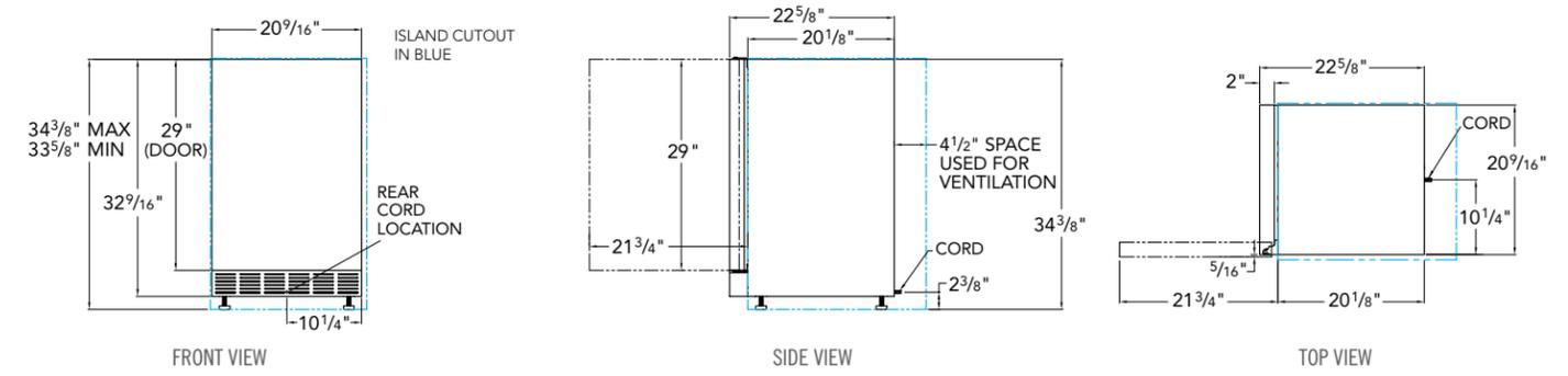
NOTE: For this illustration refrigerator has been set at a maximum height of 34 3/8"
