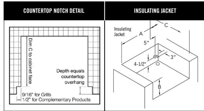
**Note:** Insulating jacket required for all grills installed into a combustible enclosure
