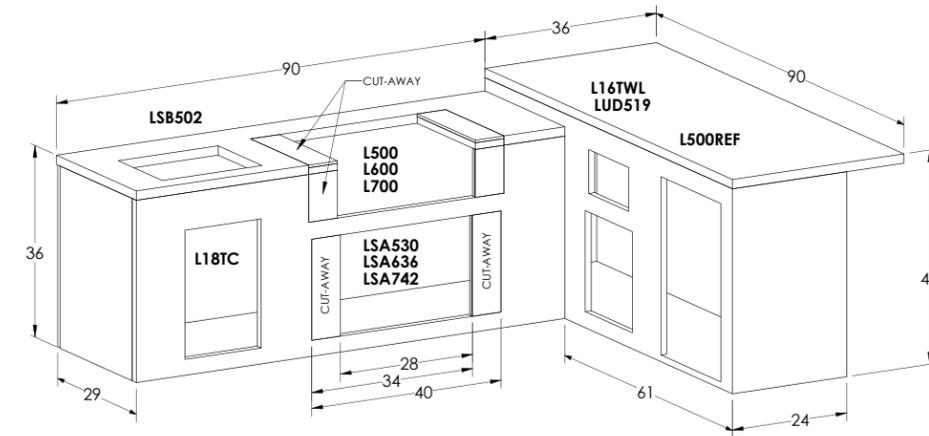
Island can be assembled 4 different ways as shown in the diagrams. Island is fully reversible. Configurations shown here:
