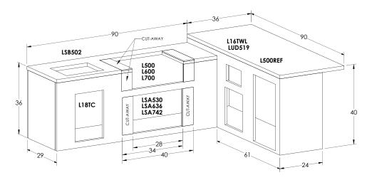
Island can be assembled 4 different ways as shown in the diagrams. Island is fully reversible. Configurations shown here:
