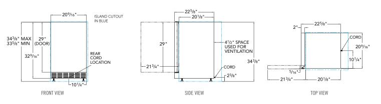
NOTE: For this illustration refrigerator has been set at a maximum height of 34 3/6"
